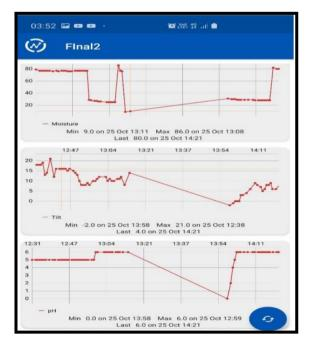
Fig. 15 - Overall Sensor Result is shown in ThingSpeak
