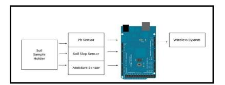
Fig. 2 - Block Diagram of the Project
