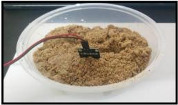
Fig. 6 - Poking the end of pH Probe into the Soil Sample
