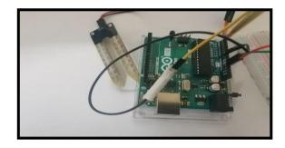
Fig. 5 - Moisture Sensor Connected to Arduino board
