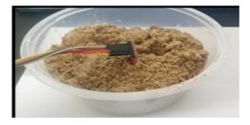
Fig. 8 - Positioning Tilt Sensor in the Soil Sample
