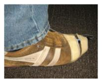
Fig. 1 - Inertial sensor attached to a shoe
