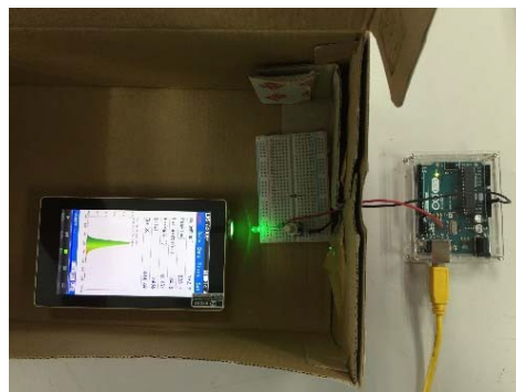
Fig. 5 - Example calibrating a 435nm LED
