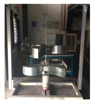
Fig. 1 - Actual photograph of the Savonius counter-rotating prototype
