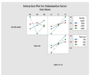
Fig. 5 - Interaction plot for delamination factor
