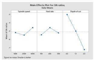
Fig.2 - Mean S/N graph for surface roughness
