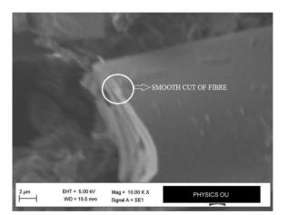
Fig. 8 - SEM micrograph showing better surface quality (Smooth cut of fibre) of CFRP composite, when spindle speed is 4000rpm, feed rate is 200mm/min, and depth of cut is 0.5mm
