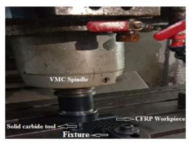
Fig.1 - CFRP composite laminate fixed in the CNC Milling machine
