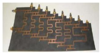
Fig. 7 - Photograph of the modified two-beam Blass matrix [25]
