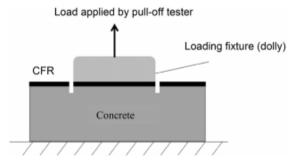
Fig. 3 - Direct tension pull off test mechanism [60]
