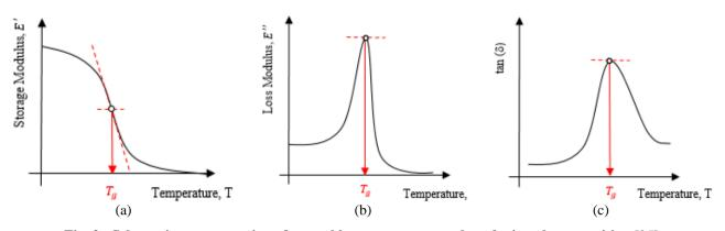
Fig. 2 - Schematic representation of several key temperature values during glass transition [25]
