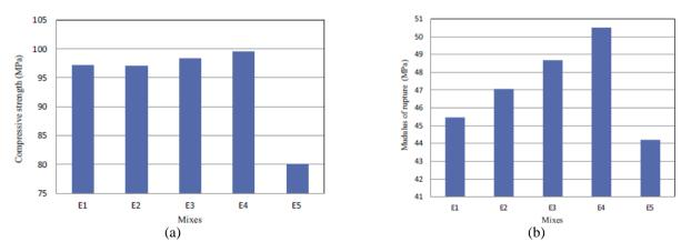
Fig. 6 - a) The effect of fine-sand ratio on the adhesive cubes compressive strength, b) The effect of fine-sand ratio to the modulus of rupture of adhesive the prisms [61]
