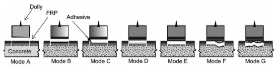
Fig. 4 - Failure modes for the pull of test [61]
