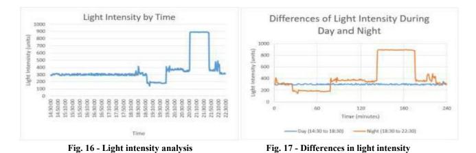
Figure 17 shows the comparison of light intensity which 4-hours during the day from 14:40 until 18.30- and 4-hours during the night from 18:30 until 22:30. During the day, the light intensity is constant at around 300 units because there is no one in the house. However, during the night the value decrease below 200 indicates high light intensity due to the LED that has been used near the plant. Then the value increases above 800 because all the light has been turned on.
