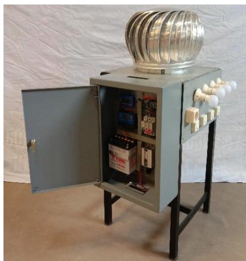
Fig. 9 - Prototype of a mini electrical power plant with a win ventilator as a turbine
