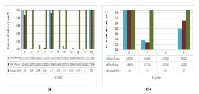
Fig. 3 - (a) The cation heavy metals concentrations of water before and after through water filter system by brand A (Model 2), and (b) The anion heavy metals concentrations of water before and after through water filter system by brand A (Model 2)
