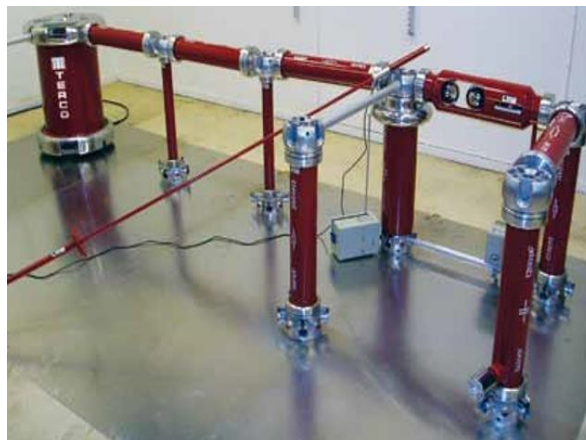
Fig. 1 - Basic single stage circuit equipment's arrangement (TERCO, 2011)
