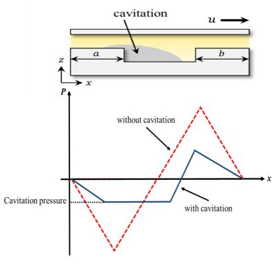
Fig. 2 - Cavitation in a single texture cell and the pressure distribution [26]
