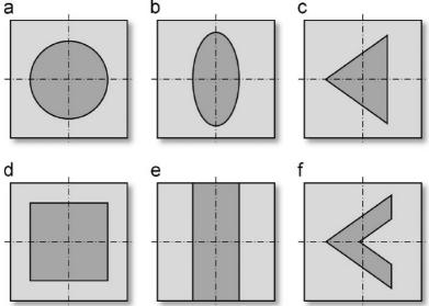
Fig. 4 - Texture shapes. (a) circular; (b) elliptical; (c) triangular; (d) rectangular; (e) groove and (f) chevron-like [26]
