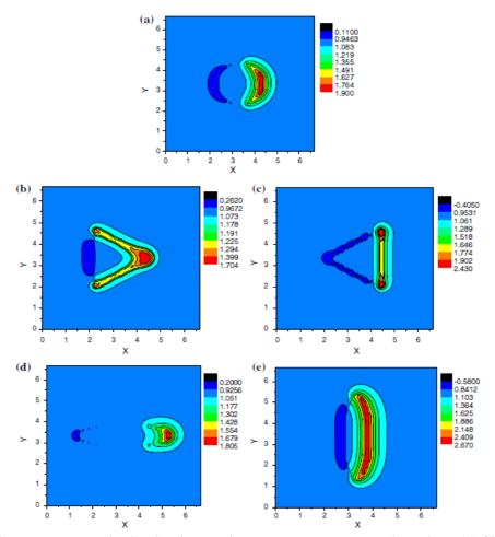
Fig. 5 - Dimensionless pressure distribution for varying textural shapes and orientations. (a) Circle; (b) Triangle (apex towards the sliding direction); (c) Triangle (apex opposites to sliding direction); (d) Ellipse (parallel to sliding direction); (e) Ellipse (perpendicular to sliding direction) [44]
