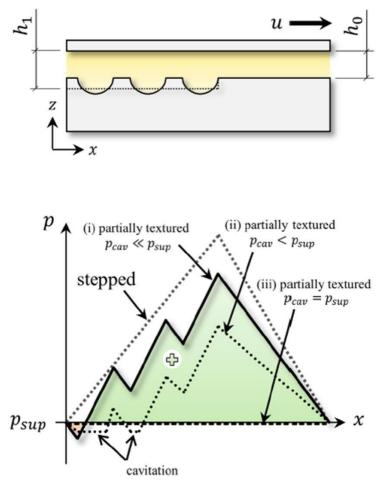
Fig. 3 - Pressure distribution overstep textured slider [26]
