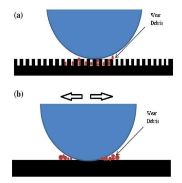
Fig. 1 - Cross-sectional view of reciprocating ball on a plate in lubricated condition. (a) Textured surface; (b) untextured surface [8]
