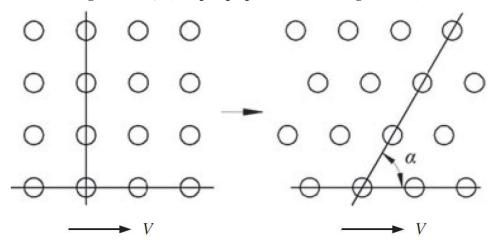
Fig. 6 - Dimple distribution array from normal square to shifted α degree array [44]
