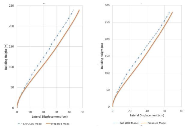
Fig. 12 - Lateral displacement profile of 60 storyhybrid system
