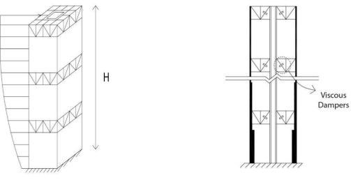
Fig. 1 - 3D model of hybrid system
