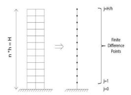
Fig. 6 - Discrete points in finite difference model
