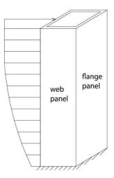
Fig. 3 - Equivalent orthotropic membrane of tubular frame
