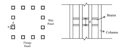
Fig. 5 - Tubular frame plan and side view for defining "b" and "d"
