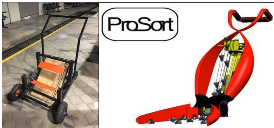
Fig. 3 - Prototype of shuttlecock collector (left); and ProSort CC-60 [43] (right)
