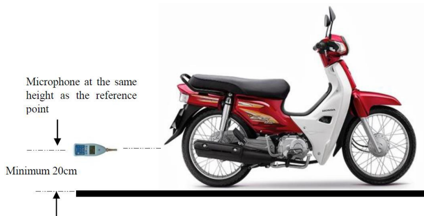
Fig. 5 - 20cm height of sound level meter to the reference point [10, 11, 14]
