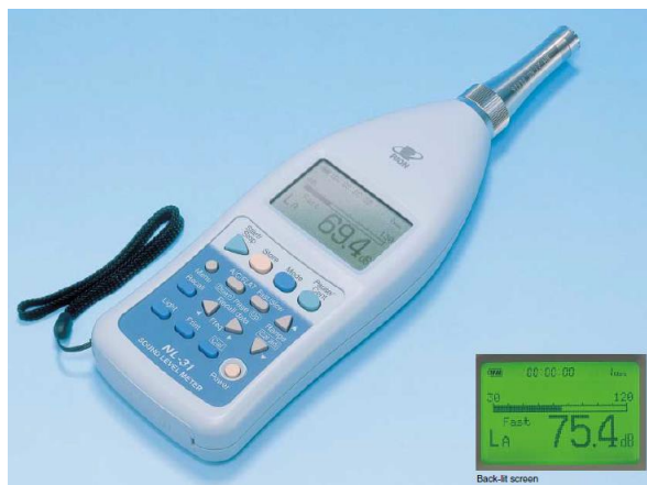
Fig. 1 - Sound level meter used in the measurement
