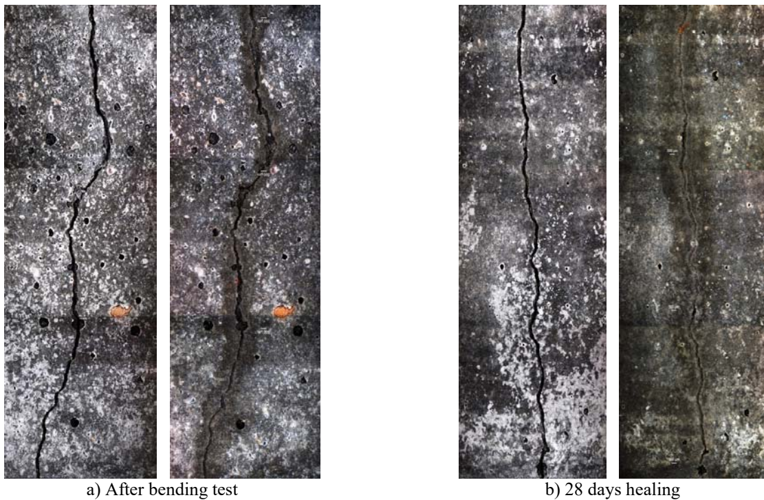
Fig. 6 - Observed of crack-healing process before and after healing treatment in control specimens by stereomicroscopy.
