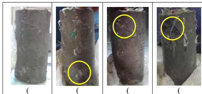
Fig. 5 - Condition of the specimens after (a) 1, (b) 2, (c) 3, and (d) 4 W-D cycles
