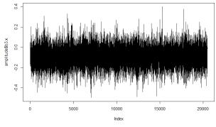
Fig. 2 - Raw vibration signal of Bearing4
