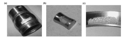
Fig. 5 - (a)Inner race failure in bearing3; (b) roller element failure in bearing4; (c) outer race failure in bearing1 (see [24])
