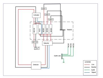
Fig. 2 - Pre-designed block diagram
