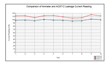
Fig. 4 - Comparison of Ammeter and ACS712 Leakage Current Reading
