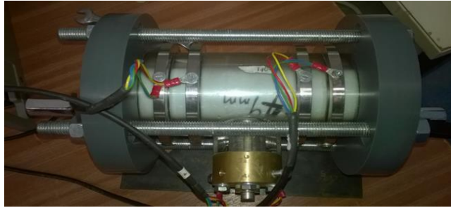
Fig. 4 - Bench annular flow calibration with both rings and probe sensors
