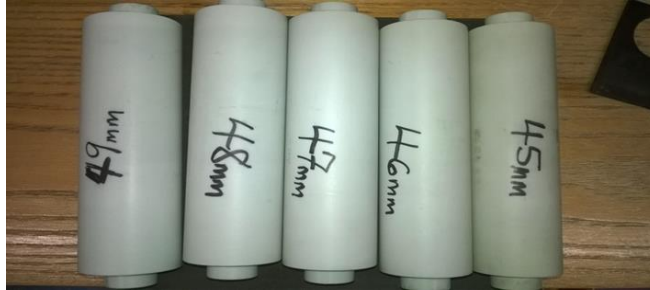
Fig. 5 - The five acrylic rods (blocks) used for annular flow calibration
