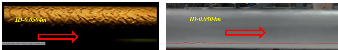
Fig. 8 - Wavy-flow of the upper pipe walls of Annular at V_{sl}=0.0901 m/s, V_{sg}=23.5707 m/s
