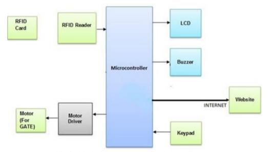
Fig. 2 - Block diagram representing the overall system
