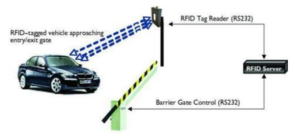
Fig. 1 - RFID barrier gate control
