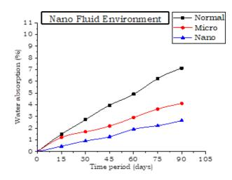
Fig. 11 - Graphical view of water absorption Vs time period under Al<sub>2</sub>O<sub>3</sub> nano fluid environment
