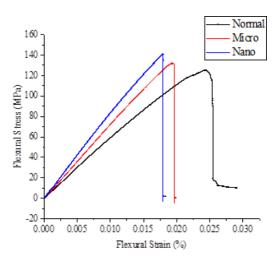
Fig. 8 - Graphical view of flexural stress Vs flexural strain
