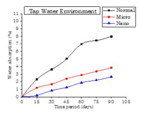
Fig. 9 - Graphical view of water absorption Vs time period under tap water environment
