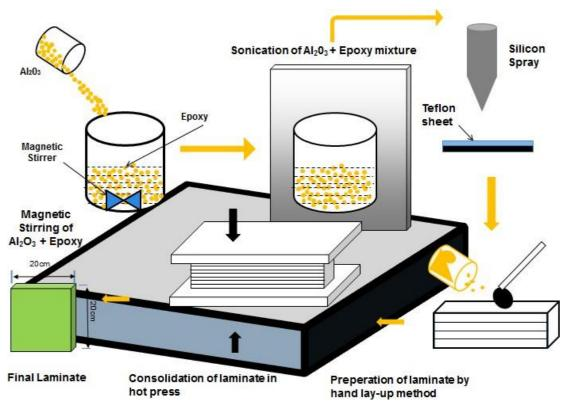
Fig. 1 - Schematic process for fabrication of composite laminate
