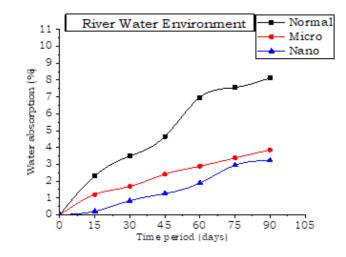
Fig. 10 - Graphical view of water absorption Vs time period under river water environment
