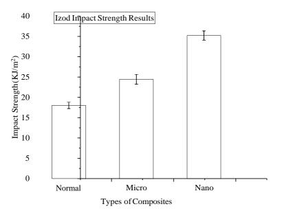
Fig. 5- Impact strength test results
