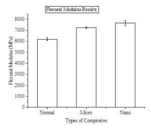
Fig. 7 - Flexural modulus results
