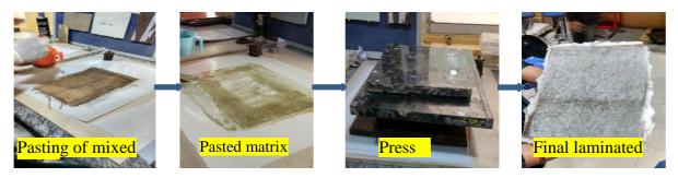
Fig. 2 - Fabrication of composite laminate
