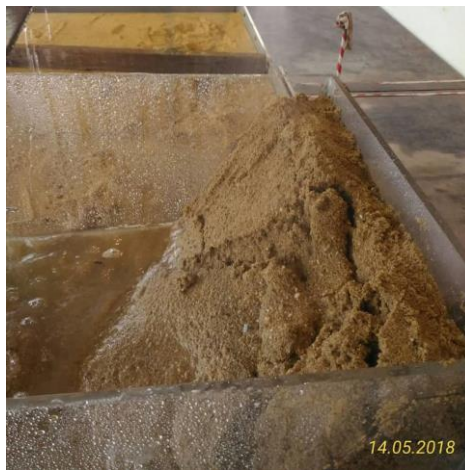
Fig. 18 - Failure of soil slope without any countermeasure.
