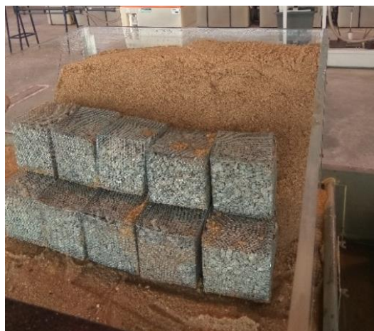
Fig. 19 - Settlement of gabion wall at the end of the rainfall test.
