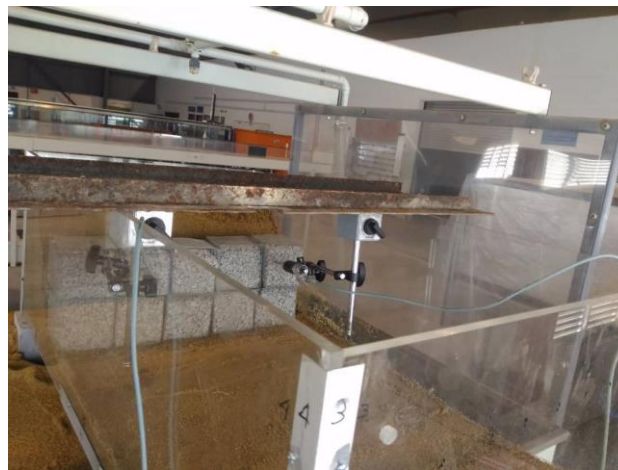
Fig. 6 - Position of the displacement transducer.
