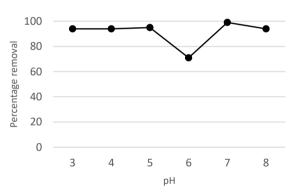
Fig. 4 Percentage removal of suspended solid of varied pH at dose PAC 3g/L.
