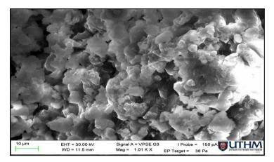
Fig. 12 - SEM image sludge leachate at dose 3g/L of PAC.
