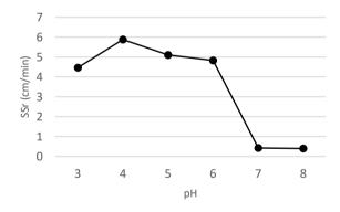
Fig. 9 - Sludge settling rate of varied pH at dose PAC 4g/L.
