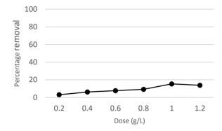
Fig. 10 - Removal of suspended solid of varied dose of tapioca flour at pH 6.
