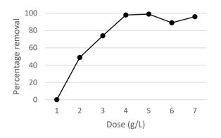
Fig. 1 - Removal of suspended solid of varied dose of PAC at pH 7.
