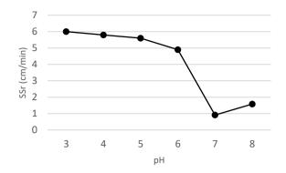
Fig. 6 - Sludge settling rate of varied pH at dose PAC 3g/L.
