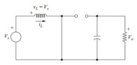
Fig. 3 - When the switch is closed.
