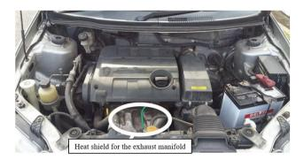
Fig. 7 - Heat source from a car.
