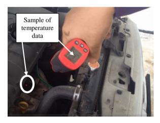
Fig. 8 - Sample of taking the temperature data using UT300A.
