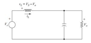
Fig. 4 - When the switch is open.
