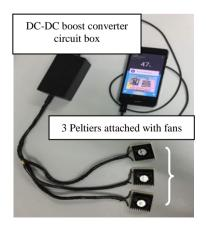
Fig. 9 - Three Peltiers and DC-DC boost converter circuit box.
