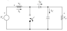
Fig. 2 - Boost converter circuit.
