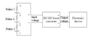
Fig. 5 - Overview of the system designed.
