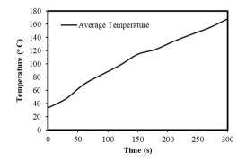
Fig. 10 - Average temperatures (°C) of the exhaust Manifold.
