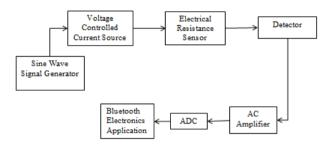
Fig. 2 - Block diagram of the system
