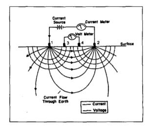
Fig. 1 - Schematic of a four-electrode resistivity measurement
