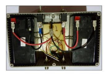
Fig. 2 - The buffer circuit to capture the lightning signal.
