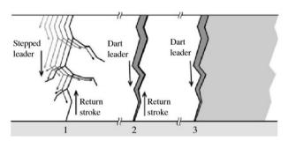
Fig. 1 - The formations of the negative cloud to ground lightning flash [8]
