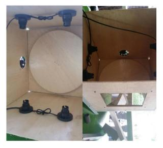
Fig. 4 - Angle view of the shoe dryer prototype.
