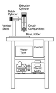
Fig. 1 - Water-powered cookies production system [14].
