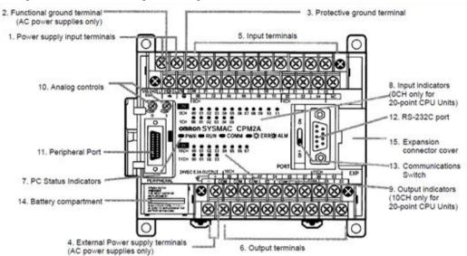
Fig. 5 - PLC unit used in the experimentation.
