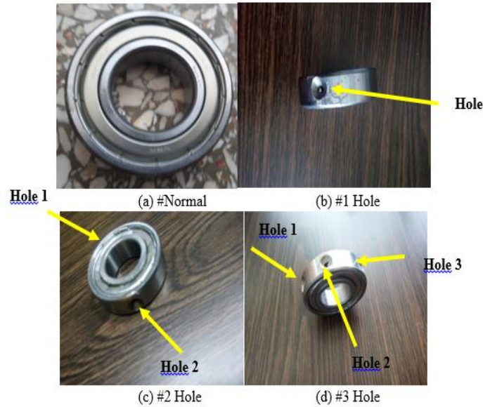
Fig. 3 - Reconstruction of outer race bearing damage
