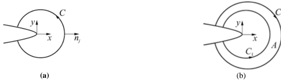
Figure 1: (a) Arbitrary contour containing the crack tip; (b) Area to calculate the J-integral
