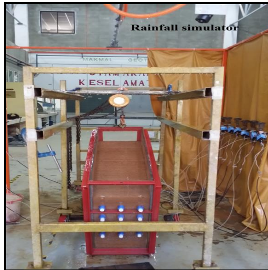
Fig. 5 - Set up for infiltration test
