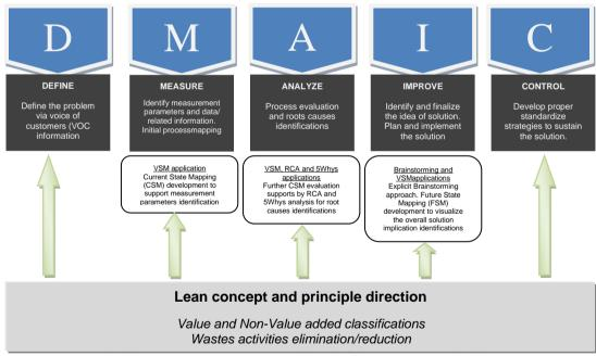
Fig. 1 – Methodology structure of DMAIC and Lean applications
