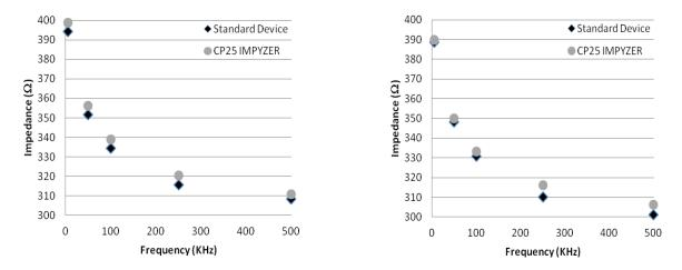
Fig. 7 - Plot represents comparative analysis of impedance measured by system prototype machine and standard device of female. (a) for Left Arm and (b) for Right Arm
