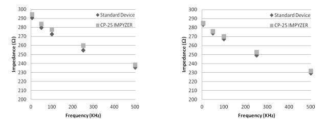
Fig. 8 - Plot represents comparative analysis of impedance measured by system prototype machine and standard device of male. (a) for Left Arm and (b) for Right Arm
