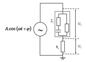
Fig. 2 - Model of bioelectrical impedance measurement
