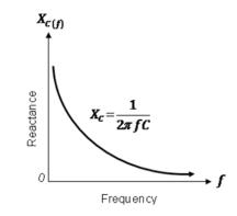
Fig. 3 – Capacitive Reactance against Frequency
