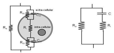
Fig.1 - (a) Model of bioelectrical impedance measurement with intra cellular water and extra cellular water; (b) Basic model of body's equivalent circuit [4]
