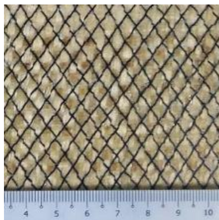
Fig. 4 - Example of stitched Tilt 60°/60° on woven kenaf fabric.
