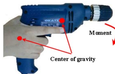
Fig. 7 – Center of gravity of tool and hand
