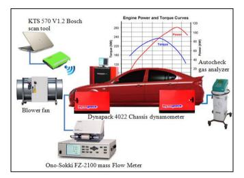
Fig. 2 Schematic diagram arrangement of engine test condition
