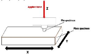
Fig. 14 Schematic drawing of Scratch Test tribometer
