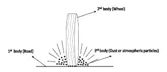
Fig. 5 Schematic drawing of a wheel and a road in contact with an introduction of dust or atmospheric particles as 3<sup>rd</sup> body (2 & 3 bodies friction)
