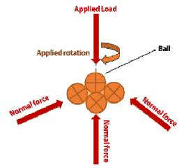
Fig. 10 Schematic drawing of a Ball on Three Balls (B3B)
