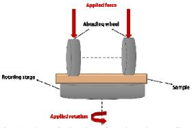
Fig. 15 Schematic drawing of a Taber Abraser tribometer.
