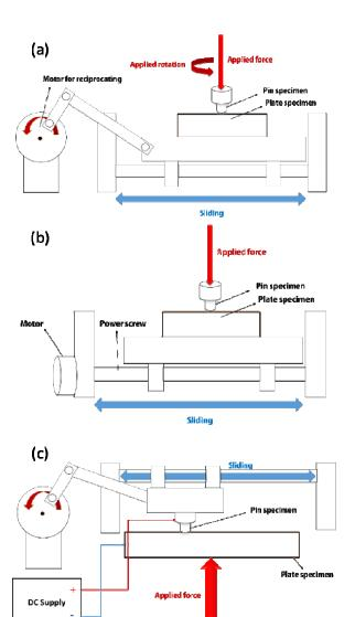
Fig. 13 (a), (b) Shows schematic drawings of possible configurations of Pin On Plate (POP) tribometer; (c) shows schematic drawing of Pin On Plate (POP) tribometer under electrification
