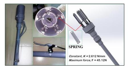
Fig. 5 - Actual design after complete fabrication process.
