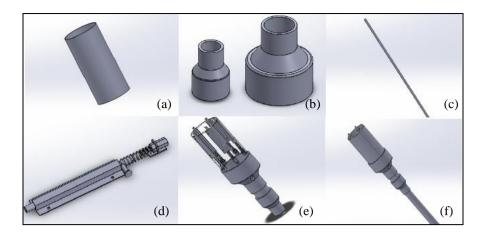
Fig. 3- Part and assembly design by using SolidWork 2016 (a) casing; (b) Connector; (c) Pole; (d) Assembly pin and spring; (e) Assembly five Jaws; (f) complete assembly all the part.
