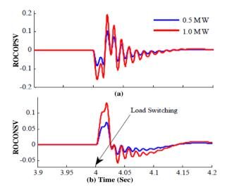
Fig. 11 - Simulation results of (a) ROCOPSV and (b) ROCOPSC for load switching
