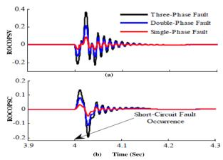
Fig. 8 - Simulation results of (a) ROCOPSV and (b) ROCOPSC during various non islanding faults
