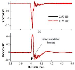
Fig. 10 - Simulation results of (a) ROCOPSV and (b) ROCOPSC during induction motor starting with different capacity
