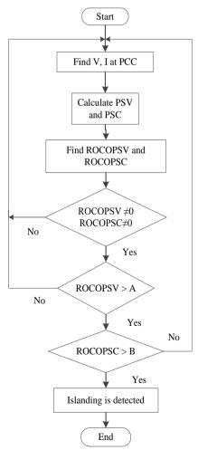
Fig. 3 - Flow chart of the proposed islanding detection scheme
