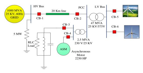
Fig. 2 - Test system under study for performance evaluation of proposed method
