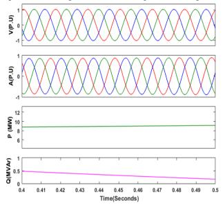
Fig.4 - Voltages, currents, active power and reactive power of grid connected operation
