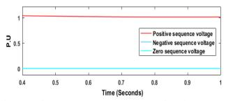
Fig.6 - Positive, negative and zero sequence voltages in grid connected operation
