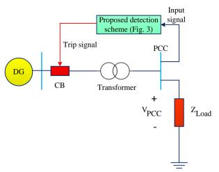
Fig. 1- Principle of islanding detection scheme
