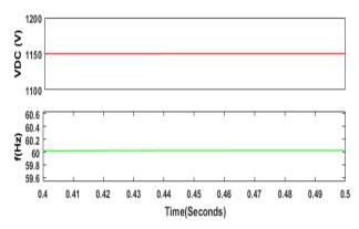
Fig.5 DC link voltage and frequency of grid connected operation
