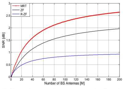
Fig. 2 SINR achieved when using many antennas M with different pilot symbols.
