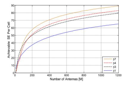
Fig. 1 Achievable SE with number of antennas *M*, for  $\beta = \{1, 3, 4, 7\}$ .
