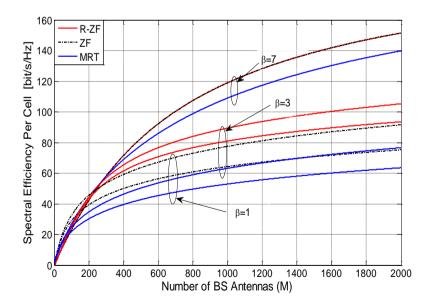
Fig. 5 Relation between the number of antennas and SE of using the pilot sequences.
