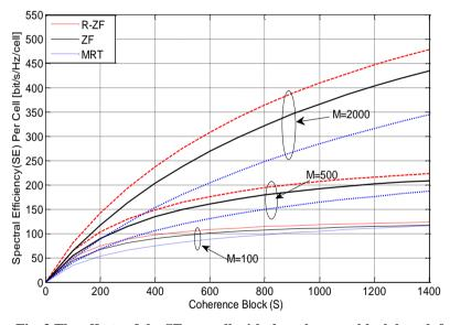
Fig. 3 The effects of the SE per cell with the coherence block length for an increasing number of antennas *M*.
