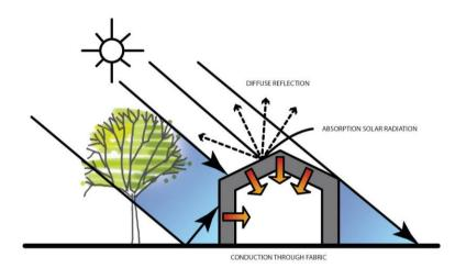
Fig. 2 – Solar heat gains through fabric
