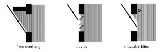
Fig. 5 - Classification of shading types
