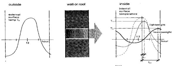
lag L decrement  $D = \Delta T_1 / \Delta T_0$  or  $\Delta T_2 / \Delta T_0$
