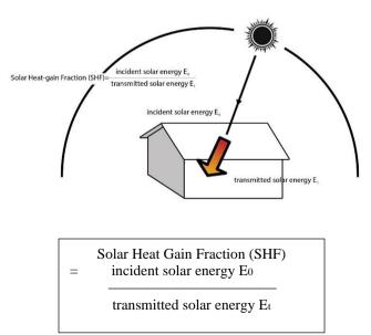
Fig. 3 - Definition of Solar Heat Gain Factors
