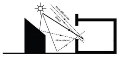
Fig. 10 – Components of light entering a room
