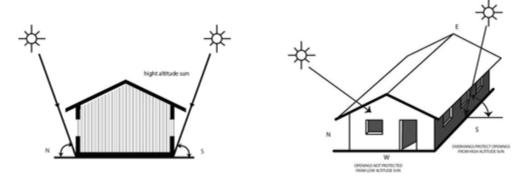
Fig. 7 - Orientation of the east and west of building to provide shading to openings in long walls
