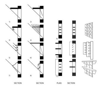
Fig. 9 - Various geometric shading devices
