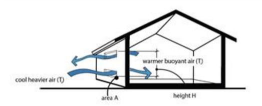
Fig. 12 – Stack Effect ventilation
