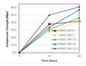
Fig 1. Compressive strength of SCC with addition metakaolin and super-plasticizer
