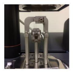
Fig. 1 Sample of PET film in tension clamp fixtures
