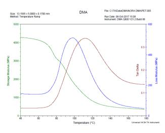
Fig. 2 Typical results of dynamic mechanical experiments of PET film from machine direction.
