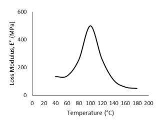
Fig. 3(b) Loss modulus of PET
