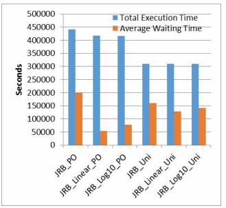
Fig. 3 - Total execution time and average waiting time using Poisson and discrete uniform distributions
