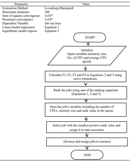
Fig. 2 - Enhanced job ranking backfilling model.
