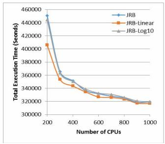
Fig. 4 - Total execution time, number of CPUs test
