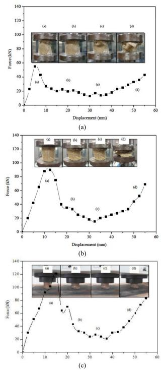
Fig. 6 Crushing mechanisms of cylindrical composite tubes (a) 2 layers, (b) 3 layers and (c) 4 layers.
