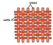
Fig. 4 A schematic diagram of woven pattern.
