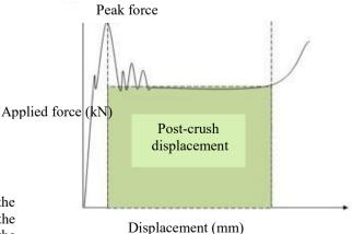
Fig. 5 Force-displacement curve.
