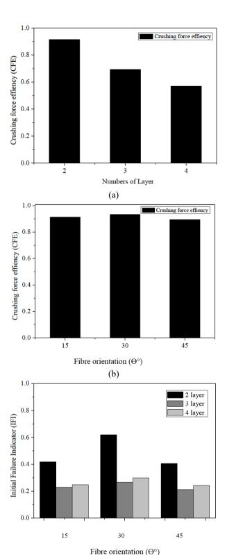
Fig. 9 Crushing performances, (a) Crushing force efficiency (effect of number of layer), (b) Crushing force efficiency (effect of fibre orientation) and (c) Initial failure indicator.
