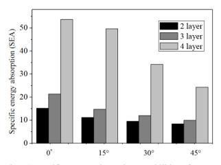
Fig. 10 Specific energy absorption capabilities of woven kenaf fibre reinforced cylindrical tubes
