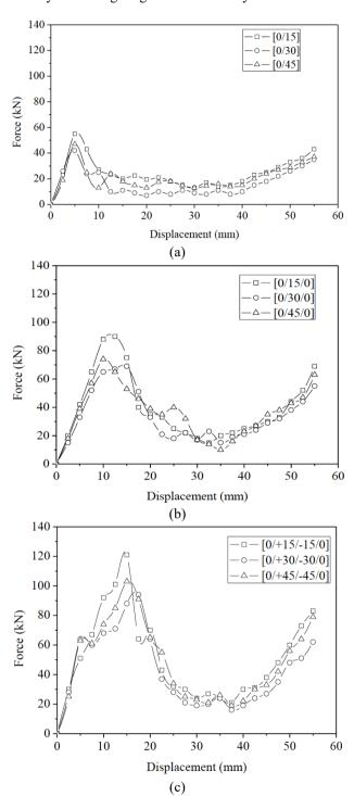
Fig. 8 Effect of number of layers on the crushing performances, (a) 2, (b) 3 and (c) 4 layers.
