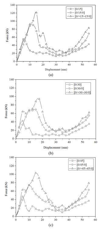
Fig. 7 Effect of number of layers and fibre orientations on the responses of force-displacement, (a)  $15^{\circ}$ , (b)  $30^{\circ}$  and  $45^{\circ}$ .
