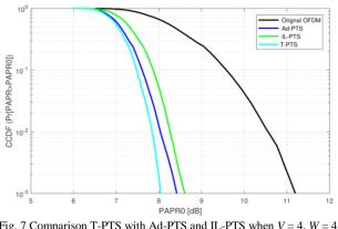
Fig. 7 Comparison T-PTS with Ad-PTS and IL-PTS when V = 4, W = 4, and N = 256
