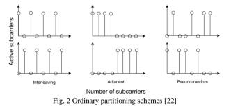
In the IL-PTS scheme, the subcarriers are assigned with equally spaced of V locations inside each subblock. The Ad-PTS scheme allots the sequential subcarriers within each subblock, successively. However, the PR-PTS scheme assigns the subcarriers within the subblocks.
