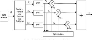
Fig. 1 C-PTS block diagram [15]
