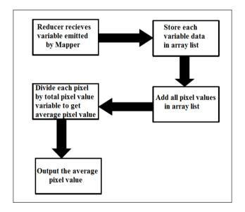
Fig. 3 Illustration of Reducer
