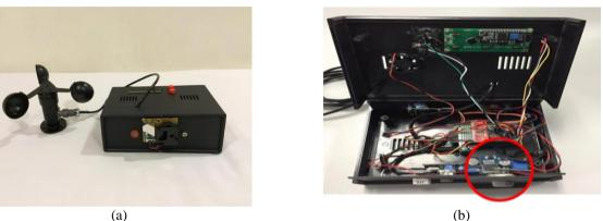
Fig. 16 (a) The system used to monitor the air pollution; (b) The internal look of the system.
