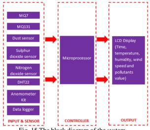
Fig. 15 The block diagram of the system.
