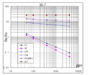
Fig. 13 The typical sensitivity characteristics of the MQ-7.
