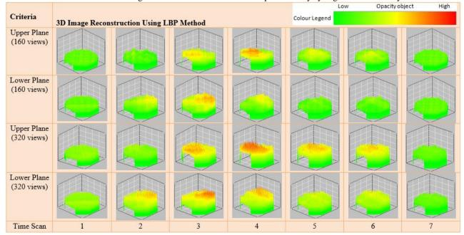
Table 1 Three-dimensional image reconstructions of air bubbles produced by syringe in LBP and Hybrid method
