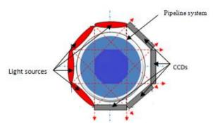
Fig. 2 CCD and laser diode sensors orientation from the top view
