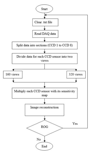
Fig. 4. Flow chart for reading real-time data for image reconstruction
